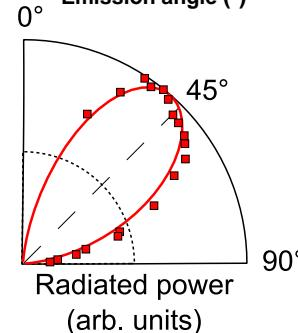
Preferential direction of emission at an angle which depends on the electronic density
