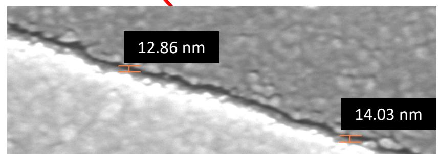
Nanotrenches width ~10 -15 nm, 33% open circuits
