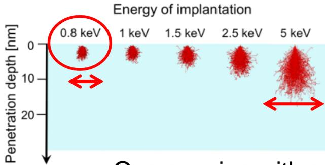
**Low energy implantation** → accurate positioning but low yield and sensitive to surface defects
