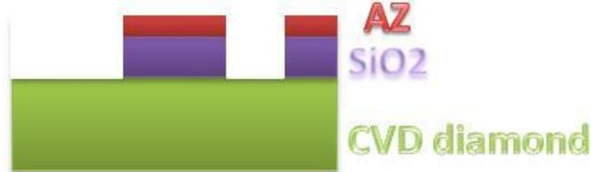
(4) Diamond ICP etching (oxygen discharge)
