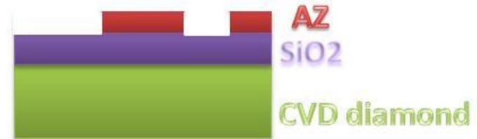
(3) SiO<sub>2</sub> ICP etching (fluorine discharge)
