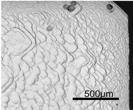
Good morphology despite presence of step bunching due to nitrogen
