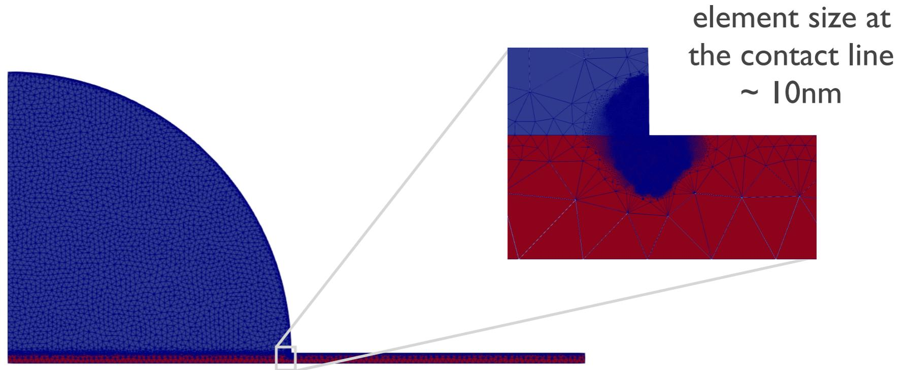
Numerical minimization of the total energy  $\mathcal{W}^I + \mathcal{W}^{II}$  is performed by a Finite Element Method under FreeFem++
