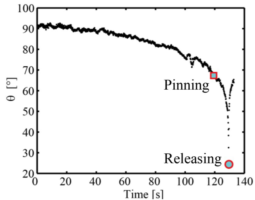
Hysteresis increases from  $\sim 5^\circ$  to  $\sim 14^\circ$  on PDMS when the drop is left at rest for 30 minutes on PDMS
