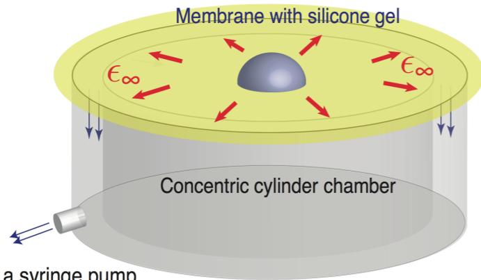
Use a syringe pump to pull the vacuum
