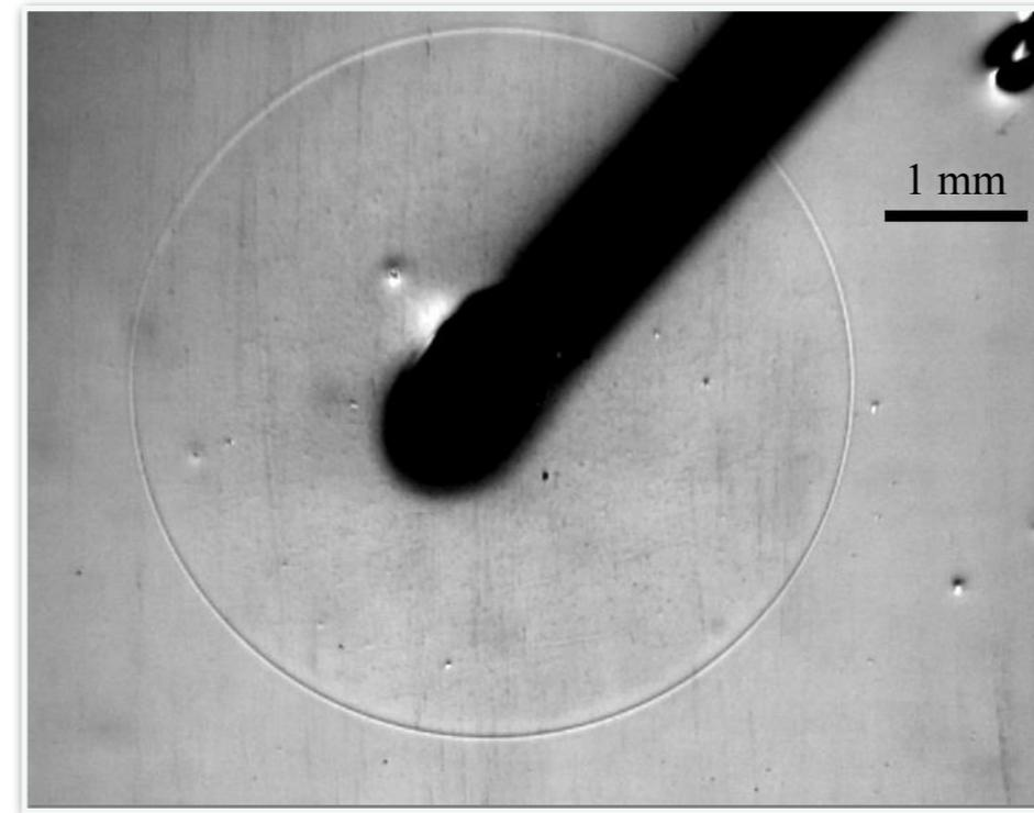
Trace left on PDMS after receding a water droplet
